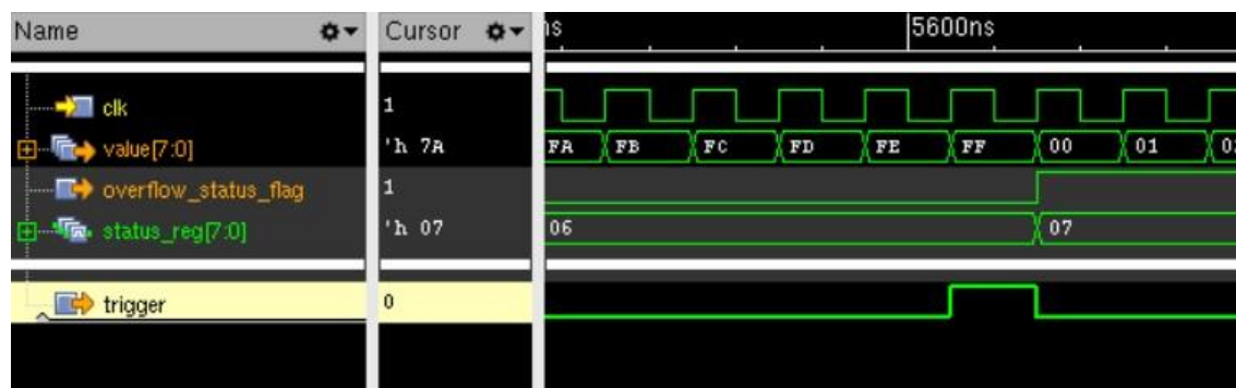
Figure 21 Trigger with overflow
