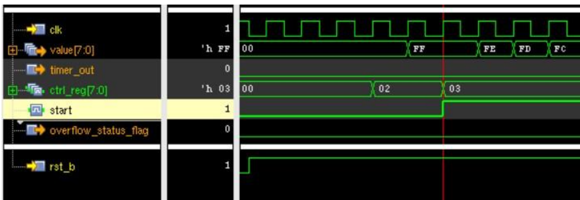
Figure 6 free run, down count mode starting
