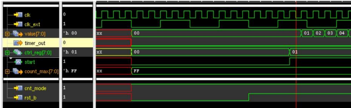
Figure 4 free run mode starting
