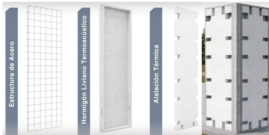
Figura 176: Detalle 3D de Panel Exterior
