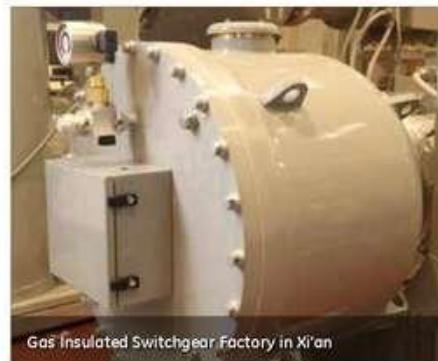
72.5kV Gas Insulated Switchgear
