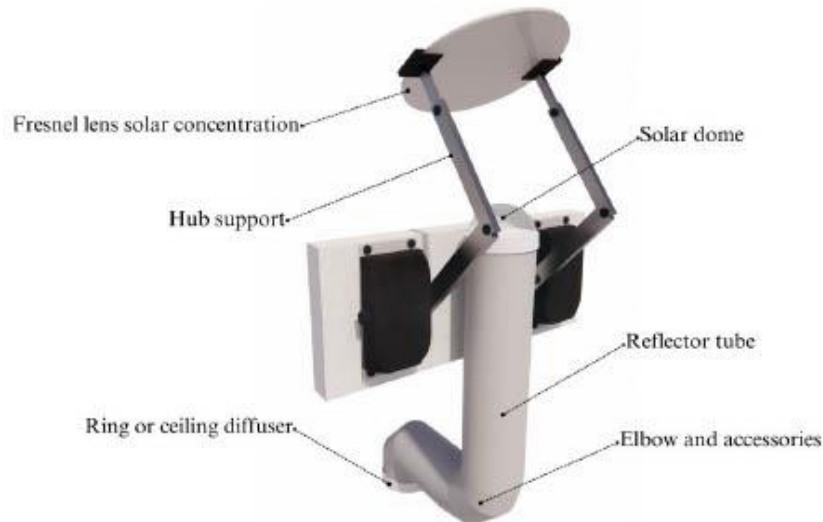
Figure 2 Design of the prototype reflector system with solar tubes.
