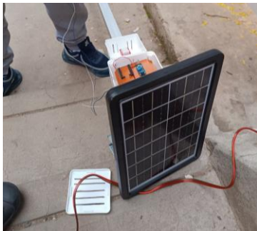
Panel solar Tx
