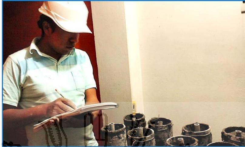
FIGURA 3.36: CONTROL DE TEMPERATURA INTERNA DURANTE 5 HORAS CONSECUTIVAS
