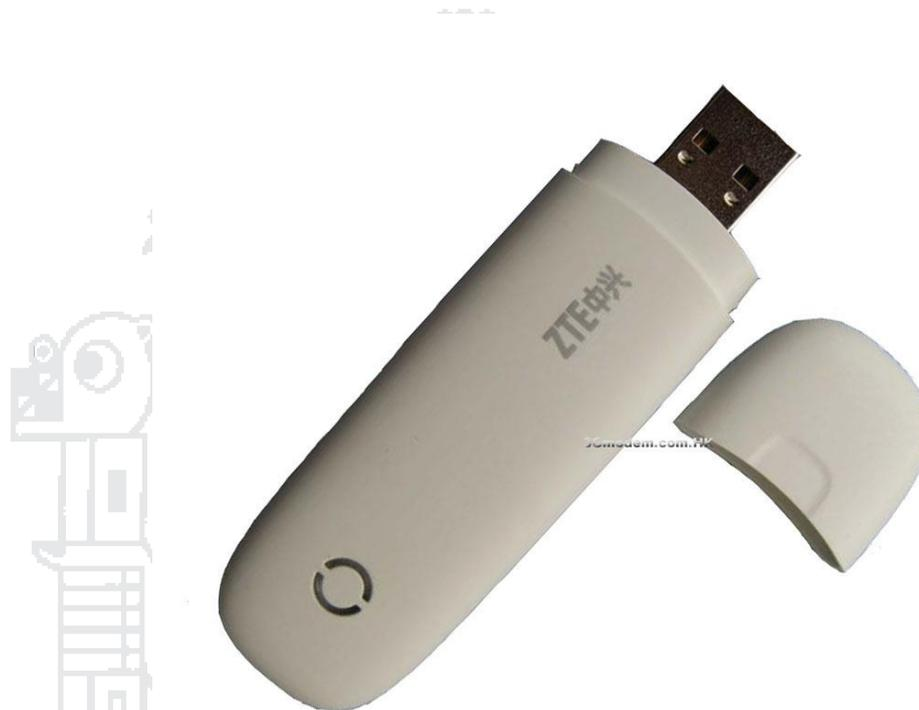
**Figura 25:** Modem USB ZTE MF180.
