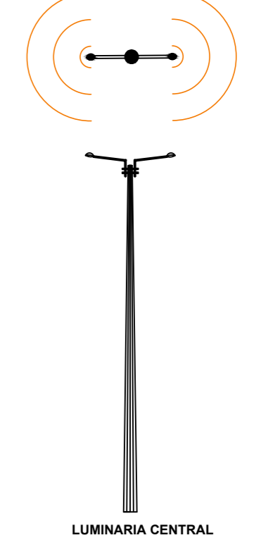
LUMINARIA CENTRAL VISTA FRONTAL
