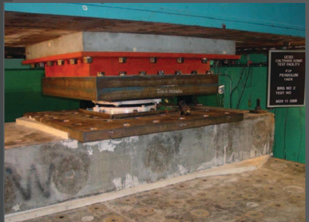
• Bi-directional type tests on a FIP-D isolator at the SRMD Test Facility at the University of California at San Diego, USA.
