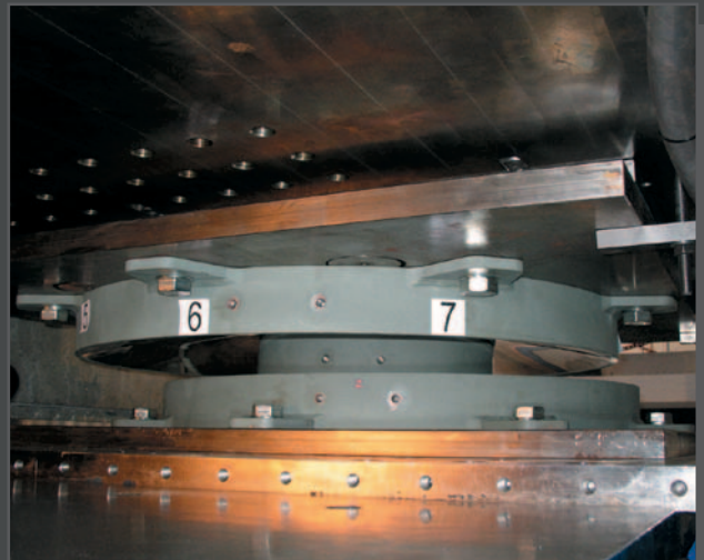
• Type tests on a double concave curved surface slider at Eucentre Trees Laboratory in Pavia.
