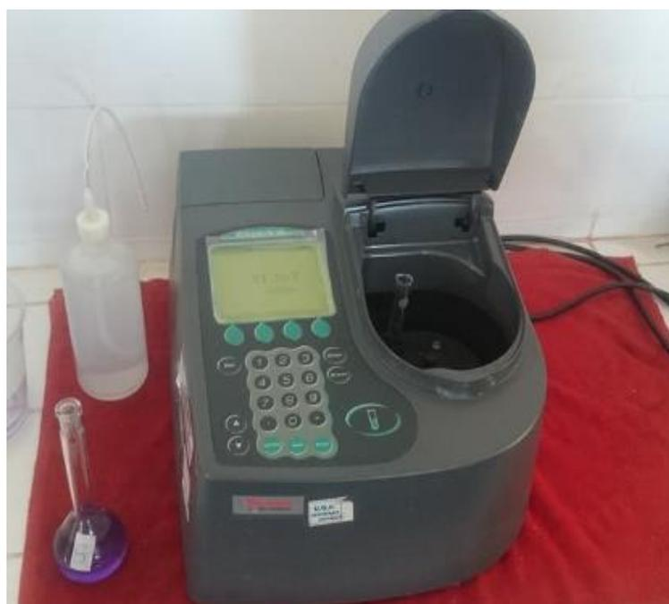
**FIGURA 5 :** ESPECTROFOTÓMETRO THERMO- SCIENTIFIC GENESYS 10S
