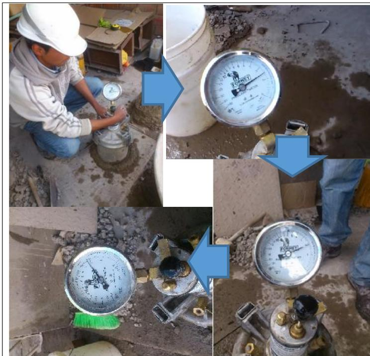
**Ilustración 49:** Contenido de aire: 12:10pm 1.2%, 12:30pm 1.5%, 13:30pm 1.9% y 14:30pm 2.3%
