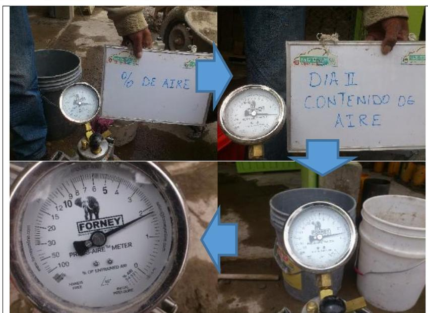
**Ilustración 48:** Contenido de aire: 09:40am 0.7%, 10:20am 1.0%, 11:20am 1.5%, y 12:20pm 1.8%
