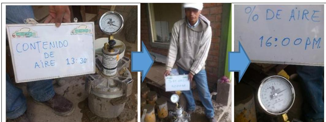
**Ilustración 47:** Contenido de aire: 13:30pm 0.6%, 14:00pm 0.8%, 15:00pm 1.1% y 16:00pm 1.4%.
