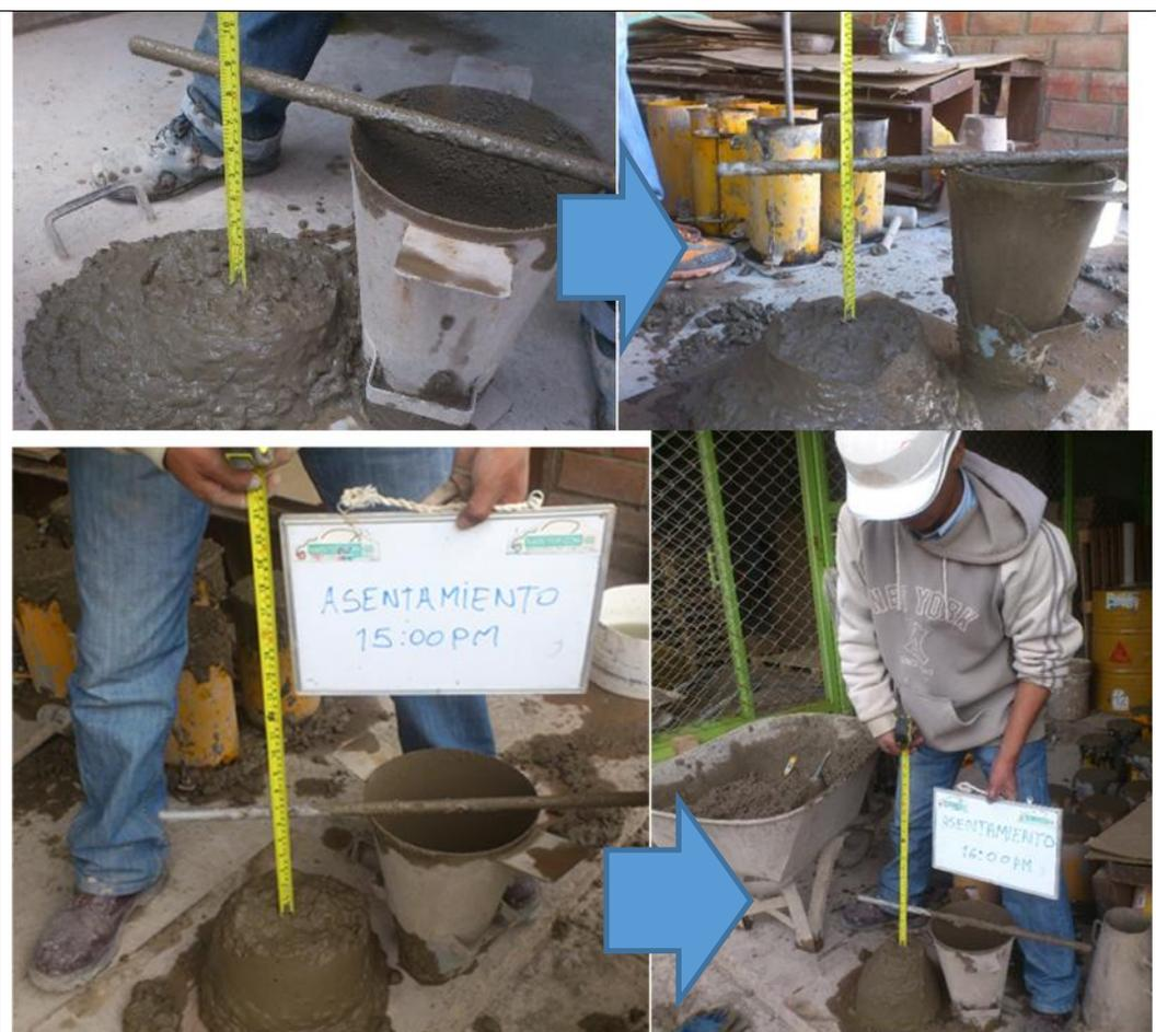
**Ilustración 27 :** Variación del asentamiento: 13:20pm Slump = 8 ¼”, 14:00pm Slump = 7 1/2”, 15:00pm Slump = 6” y 16:00pm Slump = 4”.
