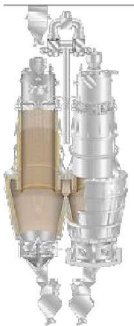
Figura 5. Horno Maerz PFR Circular
